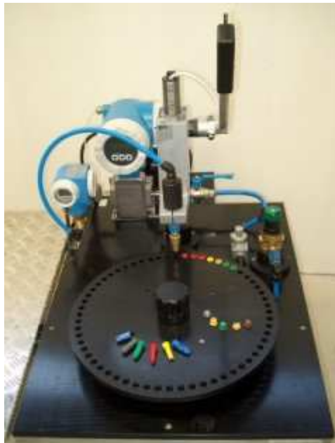
Nozzles demounted from the boom
